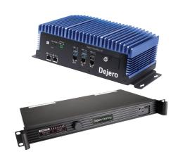
GateWay comes with 3 or 6 modems and offers rack mounted or portable, fan-less options.
